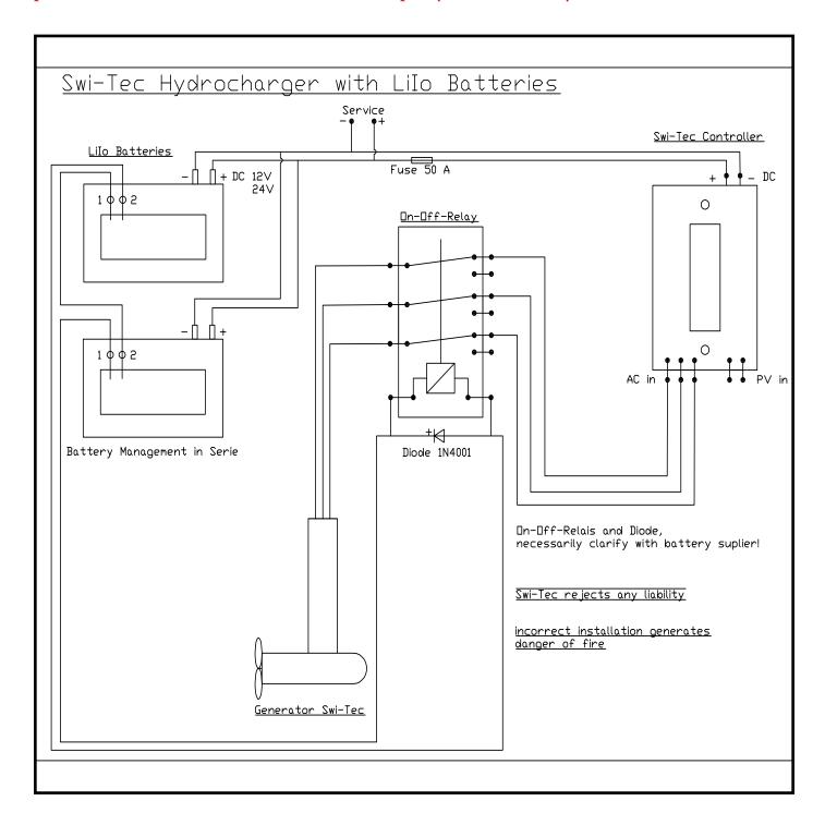
The charge controller will placed and fixed with four screws in a dry compartment in the vicinity of the batteries in a matter that you can see good the digital display. The battery cables should be as short as possible. Plus on the connector "Batt +" and with a red cable on the plus of the battery and the black cable from the "Batt –". A 40 Amp fuse in the red wire protects the HYDRO CHARGER in case of a short circuit of the batteries.
